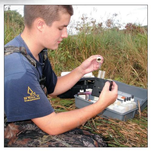
A popular water chemistry analysis kit is this model, designed for fish farmers and manufactured by Hach.
