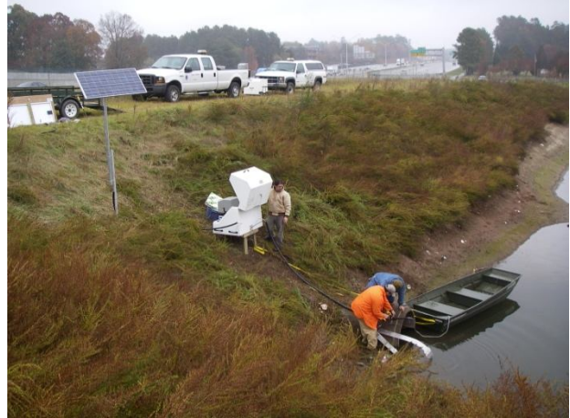
Figure 2a (left). Spring ring monitoring assembly with sample intake, suction tubing, and area-velocity meter (submerged) at inlet of Museum pond.
