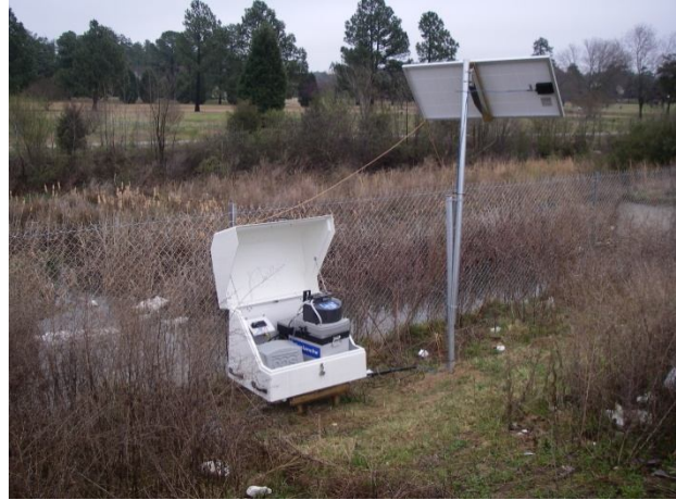
Figure 4a (left). Monitoring box containing ISCO 6712 sampler and deep cycle battery at Museum pond outlet.
