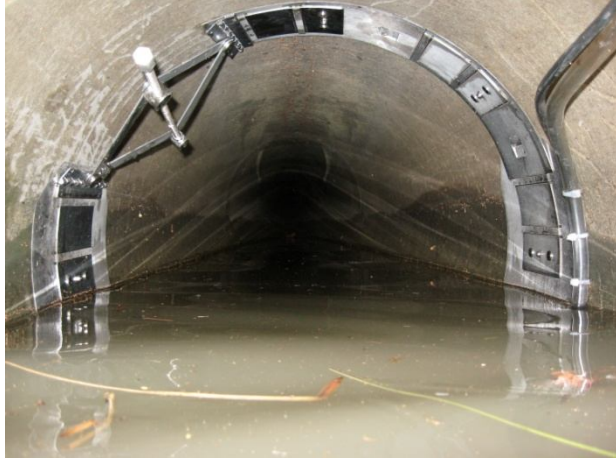
Figure 2a (left). Spring ring monitoring assembly with sample intake, suction tubing, and area-velocity meter (submerged) at inlet of Museum pond.
