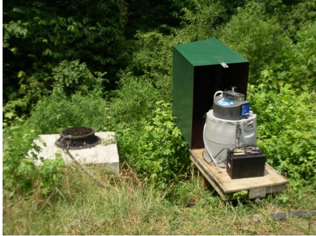
Figure 4a (left). Monitoring box containing ISCO 6712 sampler and deep cycle battery at Museum pond outlet.
