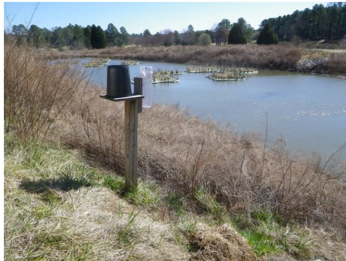
Figure 5. Rain gauge installation at the DOT pond.
