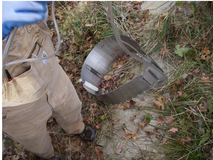
Figure 3. Spring ring monitoring assembly with sample intake, suction tubing, and bubbler assembly at outlet of Museum pond.
